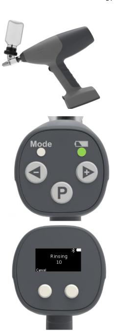
To clean the fluid path (Spike, inlet valve, cylinder, plunger and outlet valve), mount a bottle of Isopropanol or soap solution to the device and set the volume to the highest volume and do 10-20 injections to remove all residues by pressing the trigger.
