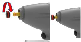
Take the piston and mount it clockwise onto the thread, don't mount it with a tool
