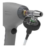
When the tube starts to fill, kink the tube just before the end to prevent loss of vaccine. Then quickly connect the tubing to the adaptor.
