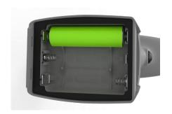
Insert the batteries in the right direction (pay attention to + and -), Before inserting the batteries check them for mechanical damage. If any damage is obvious dispose of them properly. Make sure to use the correct battery model, Please use a 18650 Li-lon PCB protected rechargeable 3,6/3,7V Batteries with a min. capacity of 2600mAh min. continuous discharge current of 5,2A to make sure you reach the product specifications.
