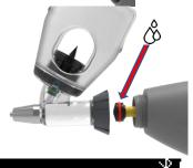
Lubricate the O-ring and then mount the new cylinder
