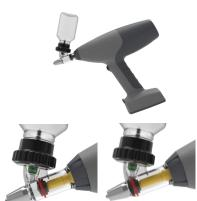
If you want to start to prime the device you can choose with the button P. The Mode will switch to the blue LED and after pressing the trigger the plunger will move to 20% of the volume for easier priming of the cylinder. Press again and the device will start to prime the device. Check the chamber if all the air is out of the cylinder.
