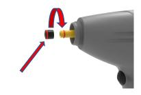
Holder piston tip and turn it counterclockwise to release it
